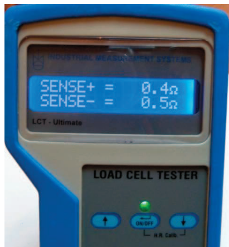
Figure 7 Typical reading when sense lines are OK
