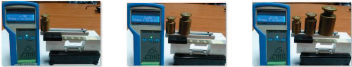
Figure 6 performing a linearity test with 3 weights
